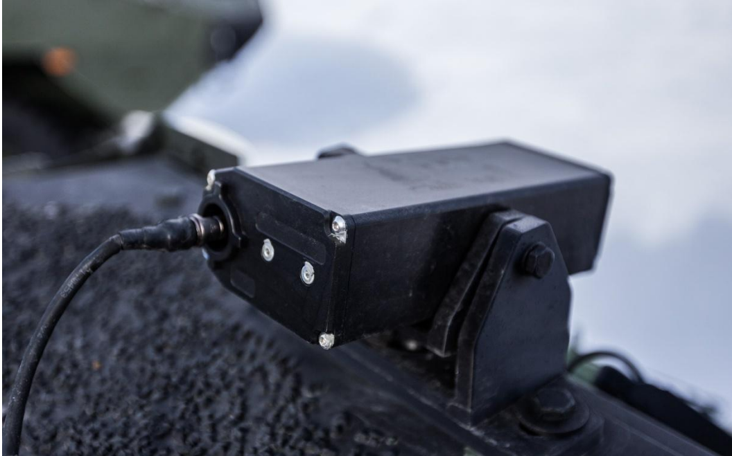
Picture 6. An Obsidian light unit assembled on the roof panel of a 6 × 6 armoured vehicle.
